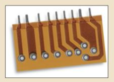
requirement, this process also supports raised solder pads above the cover layer or circuits manufactured on material as thick as .020".
